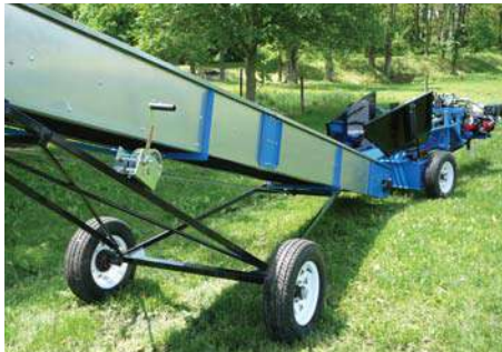
We build Elevator Conveyors up to 28' in length. Maximum height discharge is 17'.
